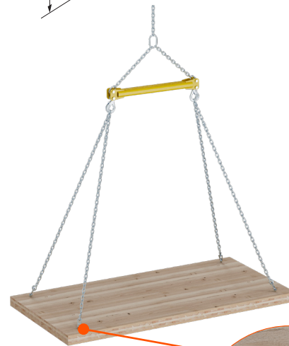
CLT Panel Rigging Using (4) MTLD Connectors
