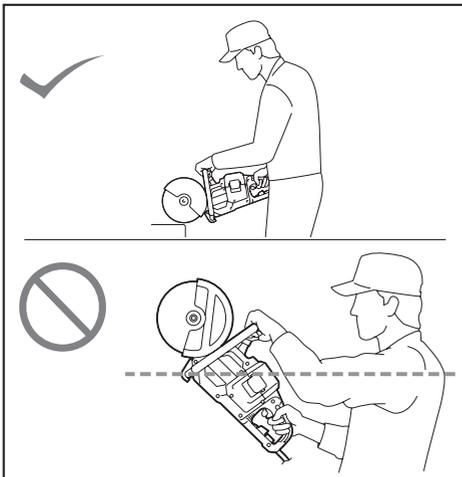
Hold the tool firmly. Grasp the handle with your right hand and the grip with your left hand. To prevent electric shock by accidental cutting of an electric cable, always hold the grip by the designated portion as shown in the figure.
