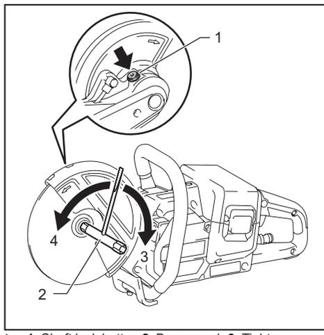
► 1. Shaft lock button 2. Box wrench 3. Tighten 4. Loosen
